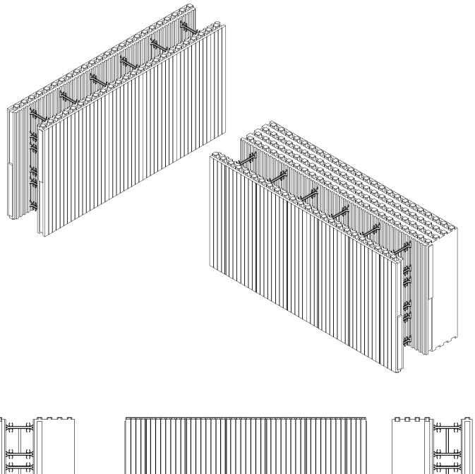
Green Isologic proposes four different blocks (Green Isologic EU, LE, PA or ZE) depending on the thickness of the external leaf.
