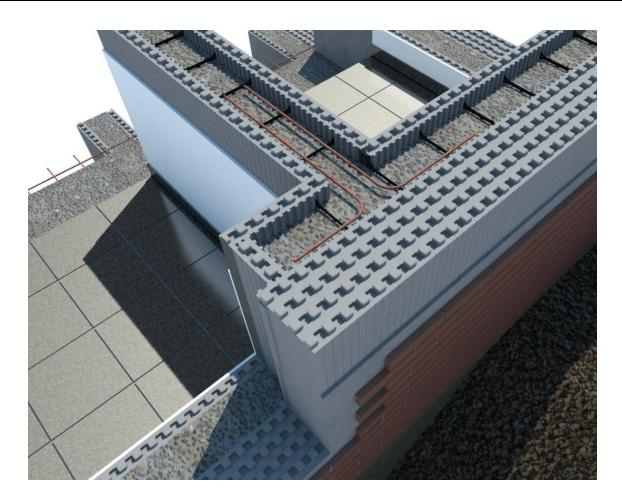
For the connection between an inner wall and an outer wall, it is necessary to cut and remove a portion of the block (inner leaf of the outer wall) to obtain a monolithic wall. Steel reinforcement can be expected to strengthen the connection.
