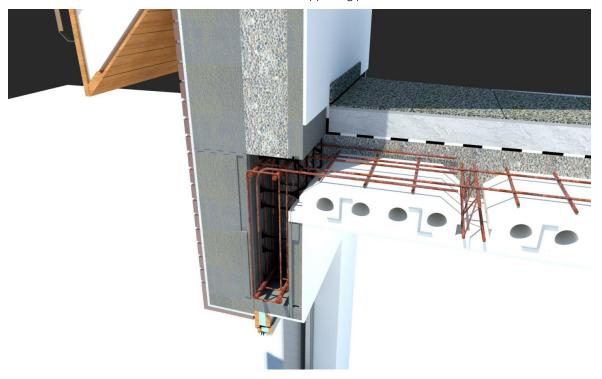
In case of precast concrete hollow core slabs
